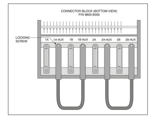
FIGURE 4-3: SUBSCRIBER BLOCK SHOWING AUXILIARY CABLING
