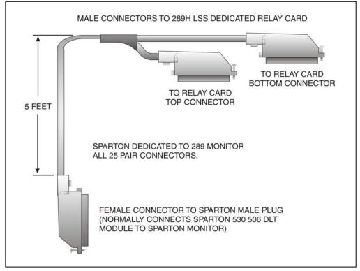
FIGURE 4-6: SPARTON TO 289H LSS CABLE
