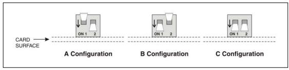
FIGURE 4-5: CONFIGURATION DIPSWITCH SETTINGS FOR SPDR
