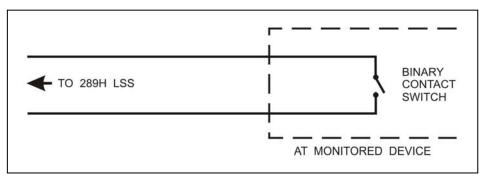
FIGURE 6-4: BINARY CONTACT WIRING
