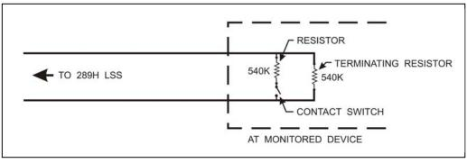
FIGURE 6-1: TYPICAL CONTACT WIRING
