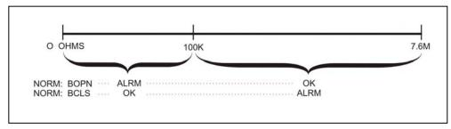
FIGURE 6-5: PAIR RESISTANCE READINGS FOR BINARY CONTACTORS
