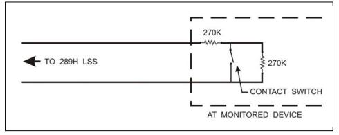
FIGURE 6-2: ANOTHER CONTACT WIRING EXAMPLE
