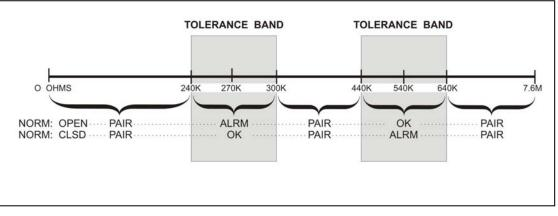
FIGURE 6-3: PAIR RESISTANCE READINGS FOR STATUS CONTACTORS
