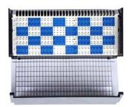
The dedicated connector block provides the means of connecting a maximum of 100 monitoring devices on dedicated pairs. Wire wrap termination pins are divided into two groups—each to accommodate 50 devices on dedicated circuits. The block is supplied with four female connectors to accommodated four 25-pair, male-to-male, cables.
