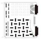
The subscriber relay card is the Loop Surveillance System's internal termination point for transducers installed on subscriber device circuits. Because of its architecture and relay configuration, it is also possible to use dedicated circuits with this card. The card accommodates a maximum of 25 devices.
