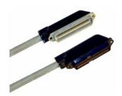
This 25 pair cable is equipped with a male and a female connector. Available in lengths from 5 to 250 feet (152 to 7620 cm), the cable is used for making the connection between a subscriber block—such as a wire wrap 9800-6056 block—and the bottom, male connector of the 289H subscriber relay card (P/N 9800-6100).
