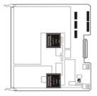
The utility card contains a 48 volt DC power supply, a micro-processor which contains the I/O circuitry for the 289H chassis, a power switch, and an alarm enable/disable switch. This card is supplied with the 289H and 289H-M monitors. It is also required when an expansion chassis is used with the 289H LSS. It provides the interface to the main chassis. The card is available here as a replacement card.
