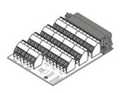
The larger, full-capacity Termination Adapter (Part No. 9010-0062) has 21 pairs of locking jaw terminals for connecting the full complement of transducers, binary devices, and the control relay pair. Once again, device numbers are printed on the circuit board to identify where the designated pairs should be terminated.
