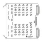
This dedicated relay card is used by the 289H/H-M monitors to read data from transducers installed on dedicated circuits. The 9800-6110 will accommodate up to 50 devices, which must be installed on dedicated conductor pairs.
