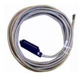
Designed for use with the System Studies Central Office Panel Rack Assemblies, the 9800-6034 cable is used to connect CO and field device circuits from termination blocks to the 289H LSS. The cable has one raw end and is equipped with a 25 pair, male connector on the other end. It can be ordered in virtually any length to accommodate individual rack assembly requirements.
