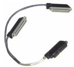
This cable makes it possible to use existing dedicated connector blocks when cutting over from a Sparton monitor to the 289H LSS. It is approximately 5 feet (152 cm) in length and has three 25 pair connectors, two for completing the connection to the 289H dedicated relay
