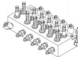
The "LSS" Flow Finder Manifold is different from the models described above in that it is supplied with stainless steel, 37° flared tubing connector fittings (to be used with braided stainless steel tubing). The "L" designation denotes the range of Flow
