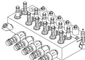
The "LBV" Flow Finder Manifold is equipped with five 0-9.5 SCFH Flow Finders (for the outgoing cable ports) and one 0-19 SCFH Flow Finder in the incoming port. Tubing connectors are nickel plated brass, 1/4" NPT to 3/8" tube, and each of the outgoing ports is equipped with a nickel plated brass check valve.
