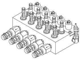
This Flow Finder Manifold is equipped with five 0-9.5 SCFH Flow Finders, one for each of the cable ports. The "BV" designation identifies the manifold's nickel-plated brass, 1/4" NPT to 3/8" tubing connectors and nickel-plated brass check valves.
