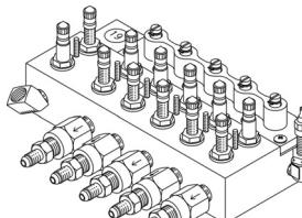
The "SV" Flow Finder Manifold contains both stainless steel, 37° degree flared tubing connectors and nickel-plated brass check valves on each of the five outgoing ports. The "L" designation represents the range of Flow Finders supplied: 0-19 SCFH (incoming port) and 0-9.5 SCFH (outgoing ports).
