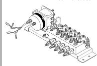
These Manifold Monitoring Assemblies are equipped with the following components: one Flow Finder Manifold with a 0-19 SCFH Flow Finder in the incoming port and 0-9.5 SCFH Flow Finders in the outgoing ports; manifold supplied
