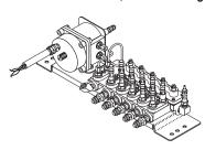
These Manifold Monitoring Assemblies include the following components: one Flow Finder Manifold with a 0-19 SCFH Flow Finder in the incoming port and 0-9.5 SCFH Flow Finders in the outgoing ports. The
