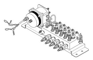
To provide ease and convenience for monitored manifold installations, System Studies provides a bracket assembly with either one or two Flow Finder Manifolds™ pneumatically connected to a High Resolution Flow or High Resolution Dual (pressure/flow) Transducer. The pneumatic connections between the transducer and the manifold(s) are accomplished by the use of two 1/8 inch (0.3 cm) stainless steel rigid tubes. These tubes are standard on all models.
