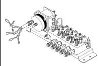
These manifold Monitoring Assemblies are equipped with one Flow Finder Manifold with a 0-19 SCFH Flow Finder in the incoming port and 0-9.5 SCFH Flow Finders in the outgoing ports. The manifold's outgoing ports are equipped with nickel-plated brass, 1/4"
