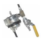
This single transducer assembly is used in a Positive Air Flow System to monitor individual cable pressure. The assembly is equipped with a stainless steel, 90-degree transducer bracket containing a 0-30 psi High Resolution Pressure Transducer. Pneumatically connected to the transducer is a branch T with a 1/4" NPT-M to 3/8" tubing
