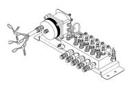
The 3902 designation identifies Positive Air Flow Return Manifold Monitoring Assemblies consisting of one PAF Return Manifold. This particular assembly uses nickel-plated brass fittings and check valves on the
