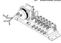
The above two assemblies are equipped with a Flow Finder Manifold with a 0-19 SCFH Flow Finder in the incoming port and 0-9.5 SCFH Flow Finders in the outgoing ports. The manifold's pneumatic tubing connectors are 37° flared,
