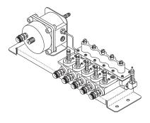
ment. It includes either one or two Flow Banks and a High Resolution Pressure Transducer™ on a rugged, easy to install, stainless steel bracket. The pneumatic connection between the pressure transducer and the Flow Bank is made using a 1/8-inch, preformed stainless steel tube.
