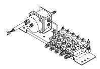
This Flow Bank Assembly consists of one Flow Bank and a High Resolution Pressure Transducer installed on a stainless steel bracket. The Flow Bank is equipped with five nickel-plated brass, 1/4" NPT to 1/4" tubing connector fittings.
