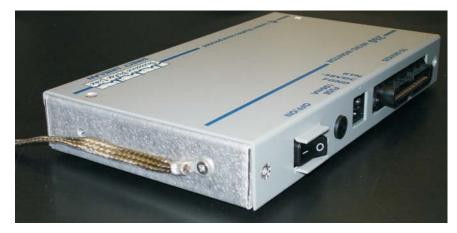
Photo 5: Repositioned Ground Strap
