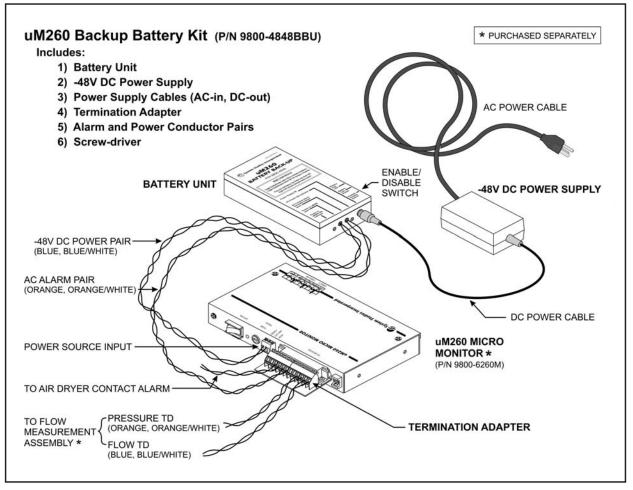
Figure 1–uM260 Backup Battery Kit Components
