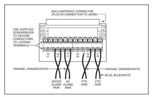
Figure 2–6-Pair Termination Adapter
