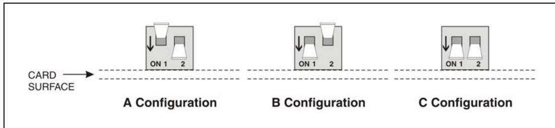
FIGURE 4-5: CONFIGURATION DIPSWITCH SETTINGS FOR SPDR
