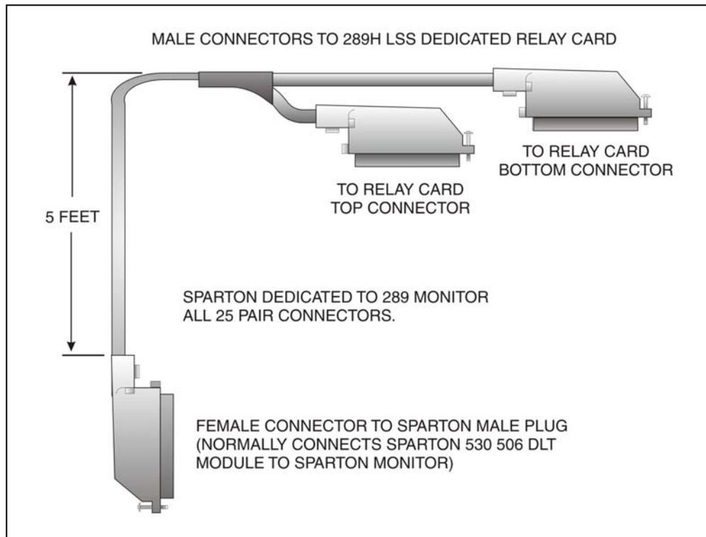
FIGURE 4-6: SPARTON TO 289H LSS CABLE
