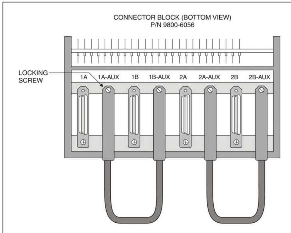
FIGURE 4-3: SUBSCRIBER BLOCK SHOWING AUXILIARY CABLING
