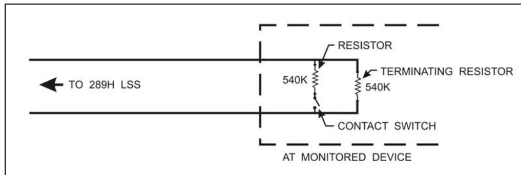
FIGURE 6-1: TYPICAL CONTACT WIRING
