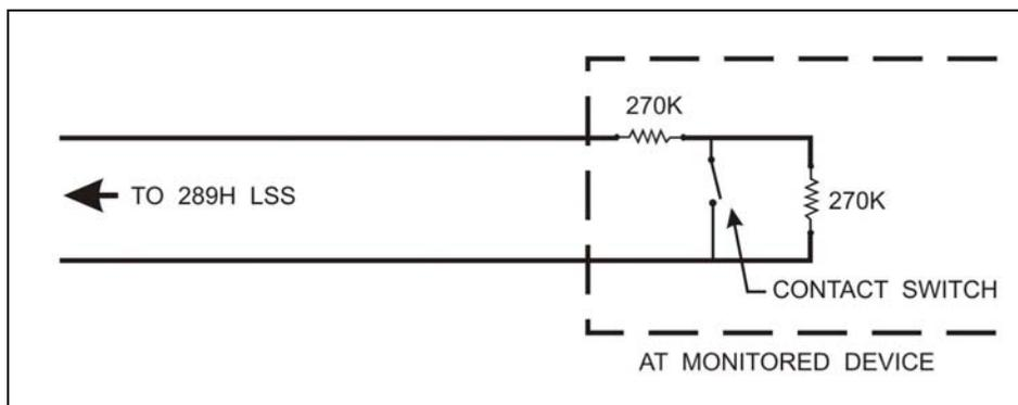
FIGURE 6-2: ANOTHER CONTACT WIRING EXAMPLE
