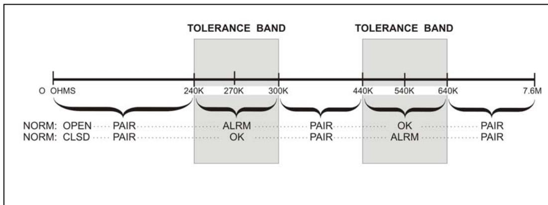
FIGURE 6-3: PAIR RESISTANCE READINGS FOR STATUS CONTACTORS
