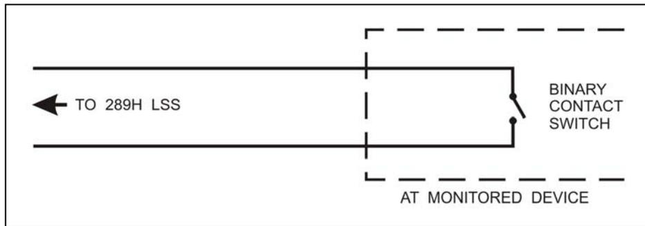
FIGURE 6-4: BINARY CONTACT WIRING
