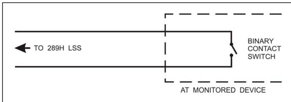
FIGURE 6-4: BINARY CONTACT WIRING
