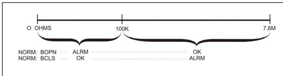
FIGURE 6-5: PAIR RESISTANCE READINGS FOR BINARY CONTACTORS
