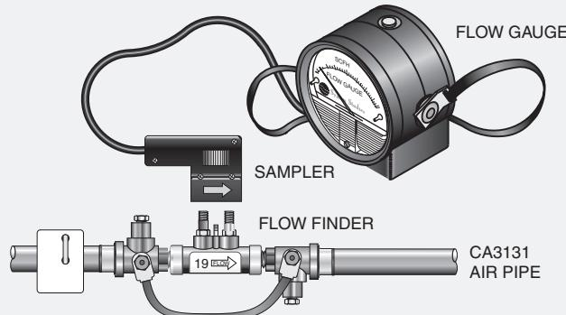
If you update your pipe routes by installing Flow Finders and Manifold Monitoring Assemblies, you can perform the following leak locating procedures with ease and accuracy: a) identify leaks, unrecorded ("ghost") manifolds, and cheater hoses, b) analyze and leak locate more efficiently, c) verify flow transducer readings, and d) verify (tag) air pipes.
