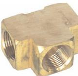
The 3/4" Union Tee is used to join three pieces of one inch air pipe. The fitting is supplied with three 3/4" NPT female threads, each of which accommodates a Power Pipe end connector (Part No. 9800-0141).
