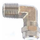
This L fitting (Part No. 6240-0008) has a 3/8" Plastic Tubing Connector with male 1/4" NPT. It is used to connect 3/8" tubing to a fitting or product equipped with a 1/4" female NPT where a 90° angle is needed.
