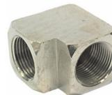
Used in Power Pipe (1" air pipe) installations, this elbow fitting makes it possible to route sections of pipe around 90° corners and/or obstructions. It is joined to Power Pipe using two Power Pipe end pipe connectors (Part No. 9800-0141).
