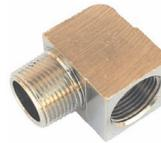
To help simplify one inch air pipe installations, particularly at locations where the pipe needs to be routed around corners, we provide a 3/4" NPT Street L fitting. This fitting is intended to be used with the Part No. 9800-0141 Power Pipe End Connector. It has a 3/4" NPT-F on one end and a 3/4" NPT-M on the other.
