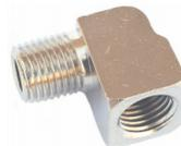
This 1/4" Street L fitting is used in a number of air pressure installations and equipment applications. It is used in the construction of System Studies' pipe and distribution panels, and in Power Pipe™ installations—particularly when connecting CA3131 air pipe to a flow limiter adapter (Part No. 9800-3035) at a Power Pipe Manifold. The fitting has a 1/4" NPT-M thread on one end and a 1/4" NPT-F on the other.
