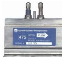
This 0-475 SCFH High Range Flow Finder is designed for use with 1" air pipe systems (Power Pipe Systems). It provides accurate flow readings up to 475 SCFH, with extended reading capabilities to 950 SCFH. This Flow Finder is supplied with mounting bracket and valves
