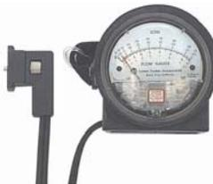
The Flow Gauge is a measurement device that converts the pressure differential created by the Flow Finder into an accurate flow reading. Using a "quick connect" sampler assembly, the Flow Gauge attaches directly to the two sampler valves located on the Flow Finder.
