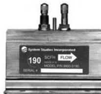
This 0-190 SCFH High Range Flow Finder is designed for use with 1" air pipe systems (Power Pipe Systems). It provides accurate flow readings up to 190 SCFH, with extended reading capabilities to 380 SCFH. The Flow Finder is supplied with mounting bracket and valves
