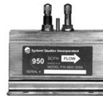
In order to monitor air dryer pressure and flow rates in a central office monitoring design, System Studies also provides a 0-950 SCFH Flow Finder. It is recommended that one of these devices be installed in both the low and high side output pipes from the air
