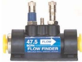
Flow Finders are equipped with an internal orifice that creates a slight pressure differential between the incoming (uphill) air flow and the outgoing (downhill) flow. This pressure differential is converted into an accurate flow reading either manually using a Flow Gauge™ or automatically by PressureMAP™ via a 289H LSS™ monitor and High Resolution Flow Transducer™.
