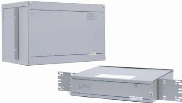
The 289H Loop Surveillance System (LSS) monitors provide a level of simplicity, versatility, and monitoring capability that is unavailable in most cable pressurization monitoring equipment. Because the 289H monitors have been designed to work with the PressureMAP™ software and utilize the MAP System™ database, they do not require expensive on-board memory and processing equipment. The result: a simpler machine with less components to break down and no need for programming or backups.
