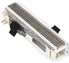
The 9800-6077-S Type 66 block accommodates 50 device pairs. It is equipped with standard punch-down, 66 clips and two 25 pair female connectors, one on each side of the block. What designates this model from the 9800-6076 and 9800-6078 blocks is the direction of the incoming cable: bottom cable entry.
