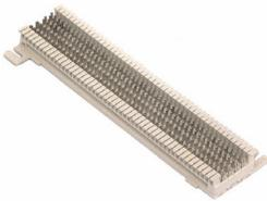
This connector block provides the means of connecting a maximum of 100 monitoring devices to the 289H/H-M using punch-down, standard clips. The block is typically used between protected blocks (P/N 9800-6062) and one of the 9800-6076, 9800-6077 or 9800-6078 connectorized Type 66 blocks described in this catalog.
