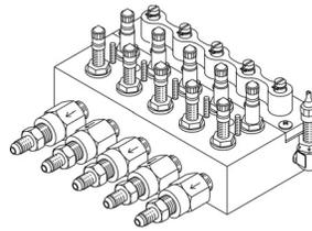
The 3070 "LSV" Flow Finder Manifold has one 0-9.5 SCFH Flow Finder in each of its five outgoing ports. It is also equipped with five 37° flared, stainless steel fittings (to use with stainless steel braided tubing) and five nickel plated brass check valves.
