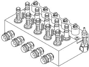
This Flow Finder Manifold is equipped with five 0-9.5 SCFH Flow Finders, one for each outgoing cable port. The manifold's "BS" tubing connectors are nickel-plated brass, 1/4" NPT to 3/8" tube. Please note that this model, and all 9800-3070 manifolds, are intended to be used
