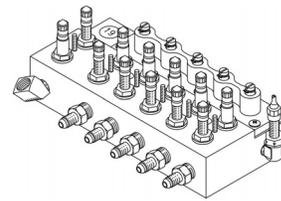
The "LSS" Flow Finder Manifold is different from the models described above in that it is supplied with stainless steel, 37° flared tubing connector fittings (to be used with braided stainless steel tubing). The "L" designation denotes the range of Flow
