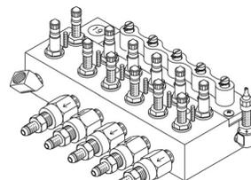
The "SV" Flow Finder Manifold contains both stainless steel, 37° degree flared tubing connectors and nickel-plated brass check valves on each of the five outgoing ports. The "L" designation represents the range of Flow Finders supplied: 0-19 SCFH (incoming port) and 0-9.5 SCFH (outgoing ports).
