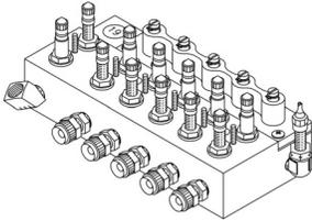
This "L" range Flow Finder Manifold is equipped with five 0-9.5 SCFH Flow Finders (for the outgoing cable ports) and one 0-19 SCFH Flow Finder in the incoming port. Tubing connectors are nickel plated brass, 1/4" NPT to 3/8" tube.
