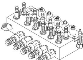
The "LBV" Flow Finder Manifold is equipped with five 0-9.5 SCFH Flow Finders (for the outgoing cable ports) and one 0-19 SCFH Flow Finder in the incoming port. Tubing connectors are nickel plated brass, 1/4" NPT to 3/8" tube, and each of the outgoing ports is equipped with a nickel plated brass check valve.
