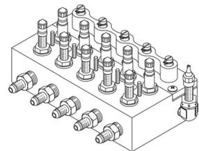
The 3070 "LSS" Flow Finder Manifold is different from the models described above in that it is supplied with stainless steel, 37° flared tubing connector fittings (to be used with braided stainless steel tubing). The "L" designation denotes the
