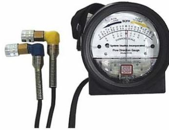
The Flow Direction Gauge is a manual air flow measurement device that provides both an accurate air flow reading and an indication of the direction of air flow. This critical information is used for leak locating in the Flow Bank System. The gauge is supplied with
