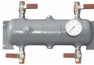
This 20-inch long, six-inch diameter air dryer balance manifold has three inlet and three outlet shutoff valves, two of which are plugged, and a 0-30 PSIG pressure gauge. It is designed to assist in accurately balancing the pressure of two or more air dryers.
