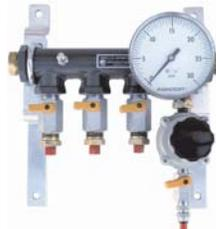
A smaller option to the 9800-5432 Balance Manifold, the 9-inch wide, 2-inch diameter air dryer balance manifold has two plugged 3/4" end inlets and four downward facing ports with shutoff valves. Also included is a large-face 0-30 psi pressure gauge and a standard tank valve. The Mini CO Manifold has two optional specifications for the four downward facing ports.
