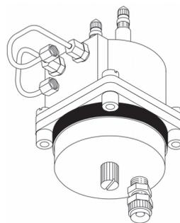
Replacement flow transducer for use on Manifold and Flow Measurement Assemblies. Equipped with nickel-plated brass connectors (side location) for 1/8" pre-formed stainless steel pneumatic tubing. Wire cover assembly supplied with nickel-plated brass fitting (bottom location) for 3/8" conductor tubing. Transducer includes 15 feet of plastic tubing and 18 feet of 2-pair conductor wire (not shown).
