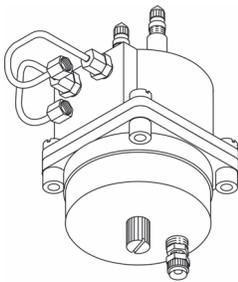
Replacement flow transducer (for use on Manifold and Flow Measurement Assemblies) equipped with nickel-plated brass fittings (side location) for connecting 1/8" preformed stainless steel pneumatic tubing. Wire cover assembly includes a nickel plated brass fitting (bottom location) to accommodate a 1/4" conductor wire tube. This model is not supplied with tubing or conductor wire.
