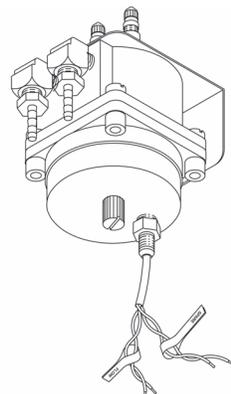
Stand-alone flow transducer equipped with 90°, barbed nickel-plated brass fittings (side location) for connecting pneumatic tubing. Wire cover assembly includes a 37°, flared, stainless steel fitting (bottom location) to accommodate braided, stainless steel conductor tubing. Transducer is supplied with 18 feet of 2-pair conductor wire.
