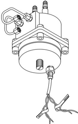
Replacement flow transducer for use on Manifold and Flow Measurement Assemblies. Equipped with nickel-plated brass connector fittings (side location) for 1/8", pre-formed stainless steel pneumatic tubing. Wire cover assembly includes a 37°, flared, stainless steel fitting (bottom location) to accommodate braided, stainless steel conductor tubing. Transducer is supplied with 18 feet of 2-pair conductor wire.
