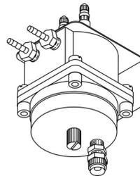
Stand-alone flow transducer with barbed, nickel-plated brass fittings (side location) for connecting pneumatic tubing. Wire cover assembly supplied with nickel-plated brass fitting (bottom location) for 3/8" conductor tubing. Transducer includes 15 feet of plastic tubing and 18 feet of 2-pair conductor wire (not shown).
