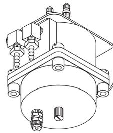
Stand-alone flow transducer equipped with 90°, barbed nickel-plated brass fittings (side location) for connecting pneumatic tubing. Wire cover assembly includes a nickel-plated brass fitting (bottom location) to accommodate 1/4" conductor wire tubing. This model is not supplied with tubing or conductor wire.
