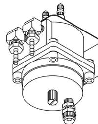
Stand-alone flow transducer with 90°, barbed nickel-plated brass fittings (side location) for connecting pneumatic tubing. Wire cover assembly supplied with nickel-plated brass fitting (bottom location) for 3/8" conductor tubing. Transducer includes 15 feet of plastic tubing and 18 feet of 2-pair conductor wire (not shown).
