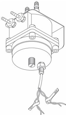
Stand-alone flow transducer equipped with barbed nickel-plated brass fittings (side location) for connecting pneumatic tubing. Wire cover assembly includes a 37°, flared, stainless steel fitting (bottom location) to accommodate braided, stainless steel conductor tubing. Transducer is supplied with 18 feet of 2-pair conductor wire.
