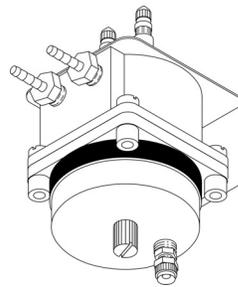
Stand-alone flow transducer equipped with barbed nickel-plated brass fittings (side location) for connecting pneumatic tubing. Wire cover assembly includes a nickel-plated brass fitting (bottom location) to accommodate 1/4" conductor wire tubing. This model is not supplied with tubing or conductor wire.
