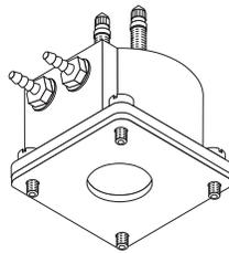
Housing mount flow transducer with barbed nickel-plated brass fitting (side location) to accommodate pneumatic tubing. No wire cover assembly or barrier plate supplied with this configuration. Intended for installation in five or ten bank, pressurized transducer housing. This model equipped with one pair of 26 gauge, stranded wire (not shown).
