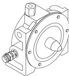
System Studies also supplies four stand-alone resistive flow transducers for use in air pressure systems that are not monitored by a 289H Loop Surveillance System. Each of the models described below provides flow readings in 40 step increments, from zero flow to its maximum rated value in Standard Cubic Feet per Hour (SCFH). In addition, they are all supplied
