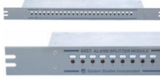
The Alarm Splitter Module makes it possible to split off 25 incoming Dual Digital Panel Meter contact alarm pairs so they can be monitored by both a 289H LSS and a secondary monitor, such as a Dantel. The rack mountable unit measures 23 inches wide (58.42 cm) by 1.75 inches high (4.45 cm) by 4.25 inches deep (10.79 cm). It contains 25 LEDs on the front of the panel to indicate which of the possible 25 pairs is in an alarm state.
