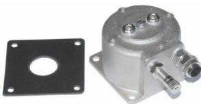
Converting from 6,000 foot to 3,000 foot manifold spacing requires installing a monitored manifold assembly at the midpoint locations. The TD housing Splice Assembly mounts directly to the existing 5-bank or 10-bank Transducer Housing at these locations and simplifies the utilization of existing pairs. It includes a tank valve and a 3/8" conductor pair tubing connection.
