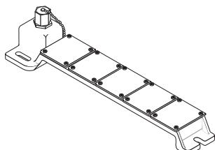
Pressure transducers monitoring cable pressure at utility hole locations are usually installed in a transducer housing. The 5 bank model, 9800-4305, is designed to accommodate up to five transducers. It is supplied with a 15 foot stub containing 6 pairs of 22 gauge PIC for cable or junction box.
