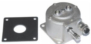
Converting from 6,000 foot to 3,000 foot manifold spacing requires installing a monitored manifold assembly at the midpoint locations. The TD housing Splice Assembly mounts directly to the existing 5-bank or 10-bank Transducer Housing at these locations and simplifies the utilization of existing pairs. It includes a tank valve and a 3/8" conductor pair tubing connection.
