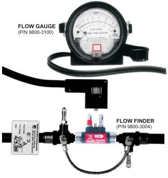
**Performance** The pressure drop across Flow Finders (all ranges) is 0.188 Pounds per Square Inch (PSI) at full air flow and 0.05 PSI at half flow. Accuracy of air flow reading is ±1% of full scale reading.
