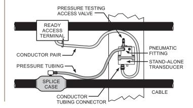
The High Resolution Pressure Transducer can be finetuned by PressureMAP to not only eliminate nuisance alarms, but provide early warning of air dryer problems.
