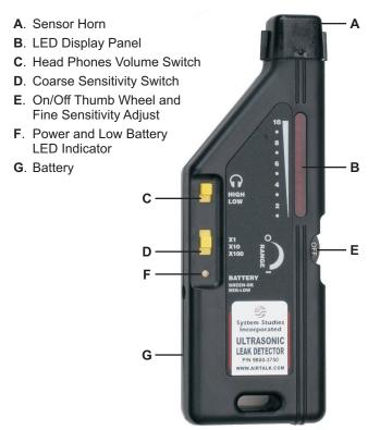
It is a simple instrument to use, as explained in the accompanying instruction sheet. A key to effectively using the device is being able to point it directly at the suspected leak. In some cases, attaching the tubing extension may provide the means necessary.
