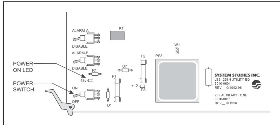
**Figure 1 - Power Switch on Utility Card**
