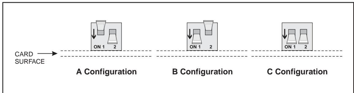
Figure 3 - Configuration Dipswitch Settings for SPDR
