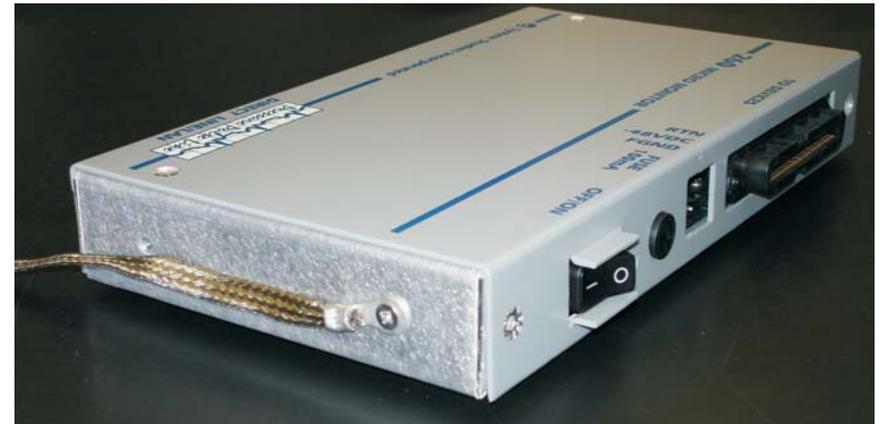
Photo 5: Repositioned Ground Strap
