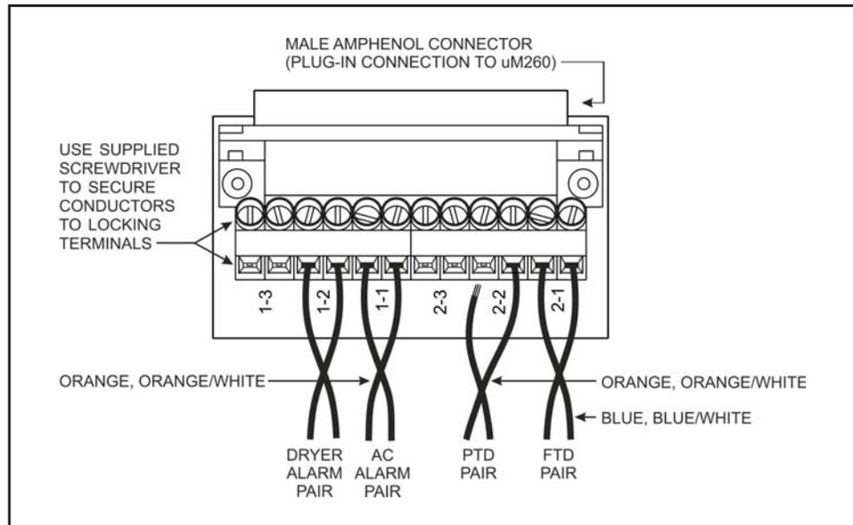
Figure 2-6-Pair Termination Adapter
