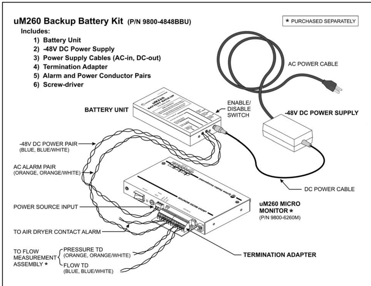
Figure 1—uM260 Backup Battery Kit Components
