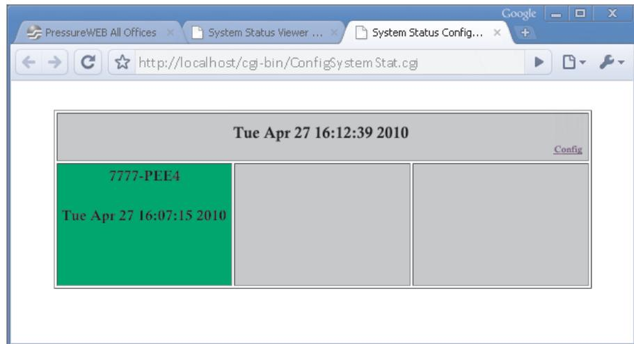
In this example, System 7777-PEE4 was the first (and only) system to report to the SSV server. As additional SSV clients are configured, reporting information will populate the other cells in this display. The first 12 reporting PressureMAP systems can be arranged on the grid using the configuration controls described in the procedures below. Additional systems will be automatically placed below them and displayed in sequence on the grid.
