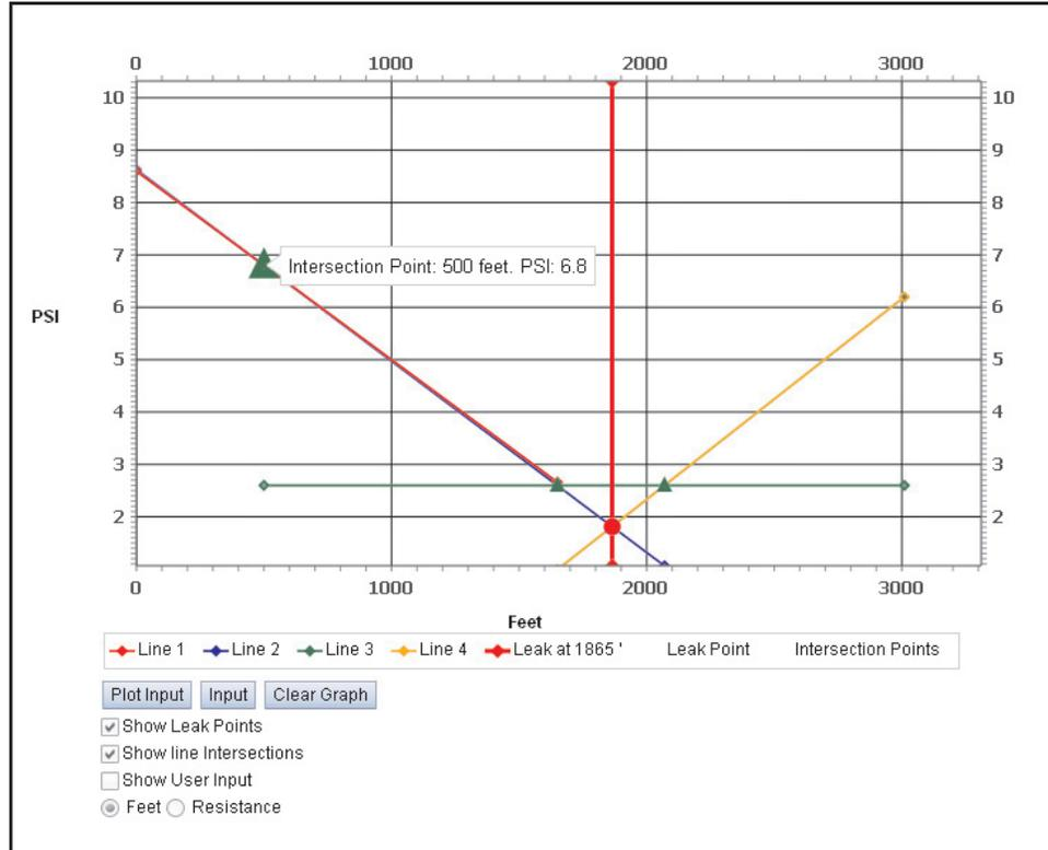
**Sample 5: Dual Feed Section, One Leak, Intersection Points Displayed**
