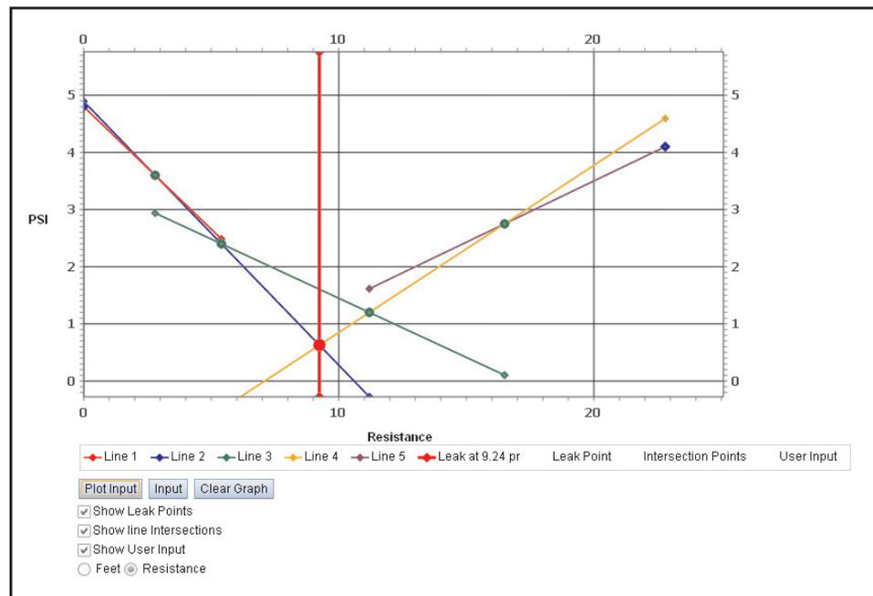
**Sample 12: Resistance/PSI Graph, Dual Feed Section, One Leak**
