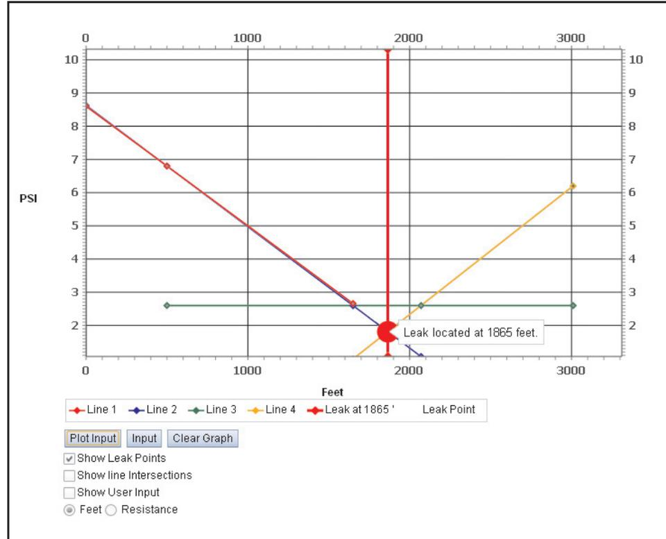
Sample 4: Graph Sample, Dual Feed Section, One Leak
